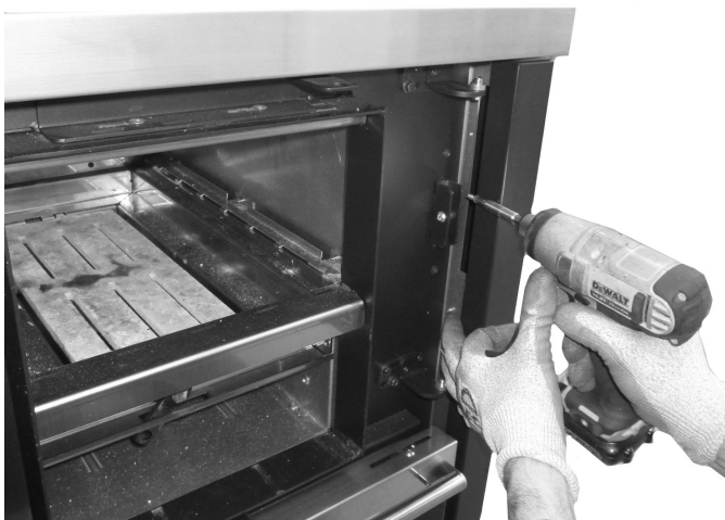
Fig. 27 - Retirer le support
