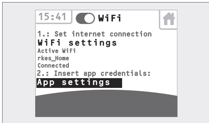
Fig. 3.33 Touch control panel – Wi-Fi receiver switched on
