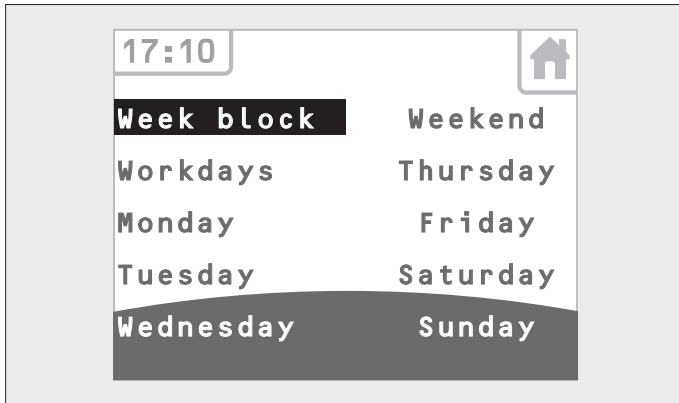
Fig. 3.23 Touch control panel – Switching times, predefined blocks of days
