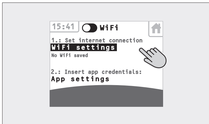
Fig. 3.32 Touch control panel – Wi-Fi receiver switched on
