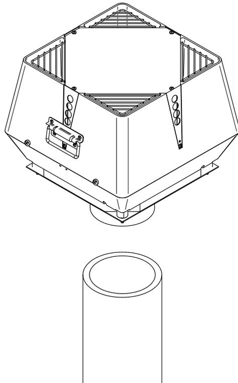
Use the safety wire to secure the fan to the chimney. Apply the supplied self-cutting screw in steel chimney. Then mount the wire through the designated hole in the base plate and into the wire lock.
