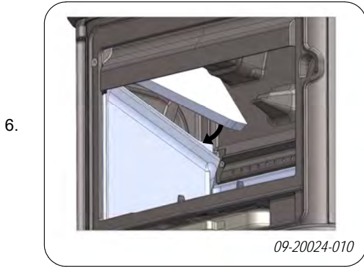
Vermiculite top Baffle plate R 03.77713.000
